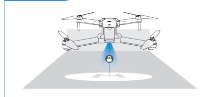
The drone is designed with an **altitude-hold** function to maintain its altitude after releasing the left joystick. (The left joystick will automatically spring back to the middle)
