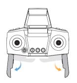
Expand the foldable handles on the transmitter separately.
