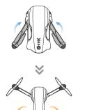
All arms of the drone are folded before the drone is packaged at the factory. First, unfold the front arms, then unfold the rear arms
