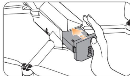
Push the battery correctly into the drone. Make sure that you hear a click sound, which indicates that the battery is firmly installed.
