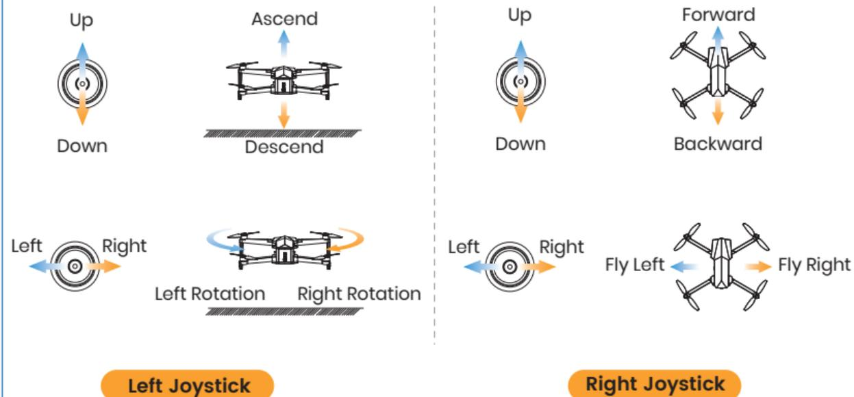
MODE 1: (Press and hold the takeoff button while powering on the transmitter to switch to Mode 1.)
