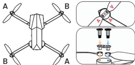
The drone will not fly unless the correct propeller is installed on the correct motor shaft. Each propeller is labeled with either an "A" or "B" on it. Secure the propeller onto the motor shaft using screws, turning each screw clockwise.
