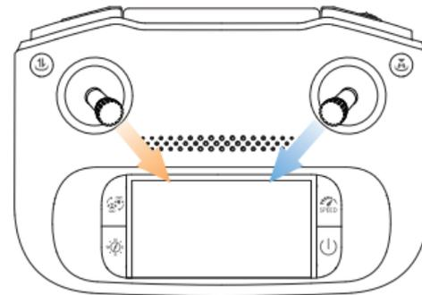
Push the joysticks towards the inner lower corners. The motors start to spin, the drone is unlocked.
