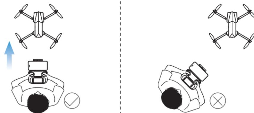
The pilot should stay facing the same direction that the drone's head points to when it takes off.
