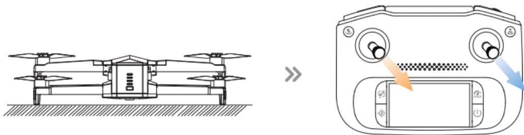
Make sure to place the drone on a level surface before calibrating the gyro. Simultaneously push the left joystick and the right joystick to the bottom right corner to calibrate the gyro. The indicator lights on the drone will blink, then turn solid, which indicates that the calibration is completed.
