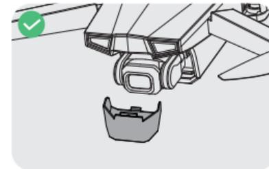
Make sure the gimbal cover is removed before the flight.
