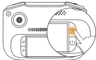
This drone offers two speed modes: Camera mode and Sport mode. Short press the
