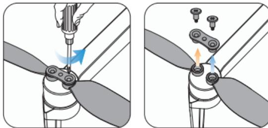
For propeller removal, use a screwdriver (provided) to rotate the screws counter-clockwise and remove the propellers. Be sure to hold the motor while detaching the propeller.
