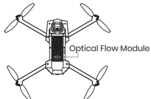
The Optical Flow Positioning System consists of a camera module, which acquires the position information of the drone through visual images to ensure precise positioning of the drone.
