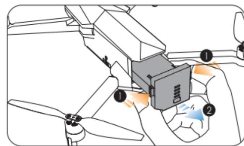
Press the lock button on the battery, and pull the battery out from the drone.
