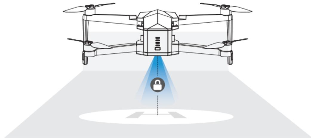
The drone is designed with an altitude-hold function to maintain its altitude after releasing the left joystick. (The left joystick will automatically spring back to the middle)
