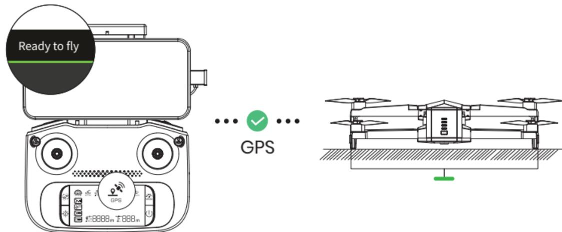
After calibrating the compass, put the drone on a flat surface. Make sure there are no external sources of signal interference around.
