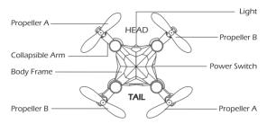
**Attention:** Pay attention to the "A" or "B" printed on each propeller. The drone will not fly unless the correct propeller is installed on the correct motor shaft.
