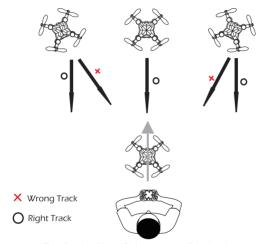
The pilot should stay facing the same direction that the drone's head points to when it takes off.
