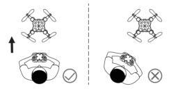
The pilot should stay facing the same direction that the drone's head points to when it takes off.
