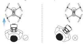
The pilot should stay facing the same direction that the drone's head points to when it takes off
