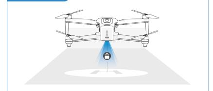
The drone is designed with an altitude-hold function to maintain its altitude after releasing the left joystick. (The left joystick will automatically spring back to the middle)
