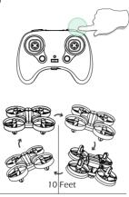
When you get familiar with all the functions of the drone, you can try this amazing flip mode. When you fly the drone at least 10 feet, press the 360° Flip button on the upper right of the transmitter, then push the right joystick Forward/ Backward or Left/ Right, and the drone will do a flip towards the corresponding direction.
