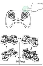
When you get familiar with all the functions of the drone, you can try this amazing flip mode. When you fly the drone at least 10 feet, press the 360° Flip button on the upper right of the transmitter, then push the right joystick Forward/ Backward or Left/ Right, and the drone will do a flip towards the corresponding direction.
