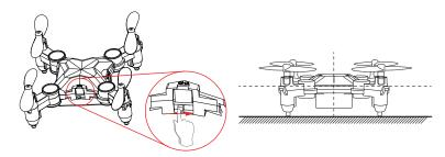
② First, slide the "Power Switch" button right to turn on the drone. Then, place the drone on flat and level surface with the head facing forward and the tail facing towards the pilot.
