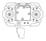
(3) Then, trun on the Transmitter. One second later, one beep will be heard and the drone's indicator lights will start flashing and then turn solid, indicating that the drone and the transmitter have been paired successfully and automatically.
