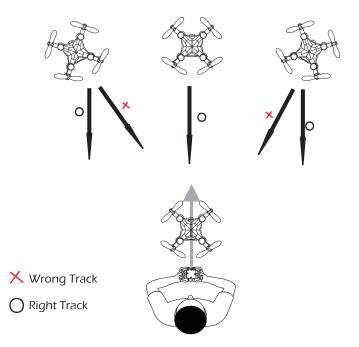
With a press of the One Key Return button, the drone will return along the parallel direction where the tail of the drone pointed to when the drone was paired.
