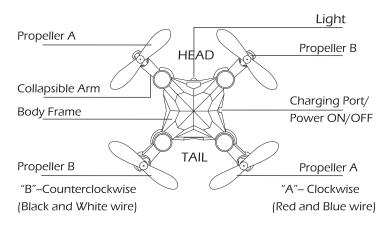
Please note that all propellers must be installed in the correct orientation.(Pay attention to the letter "A" or "B" printed on each propeller when installing.)
