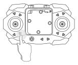
(6) Press One Key Take-off button, the drone will take off auto--matically. Or push throttle(left) joystick up slowly to take off and ascend the drone.
