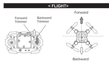
① Forward/ Backward Sideward Fly Trim: When the drone drifts forward, press the backward trimmer button to rebalance the drone; if the drone drifts backward, press the forward trimmer button to rebalance the drone.
